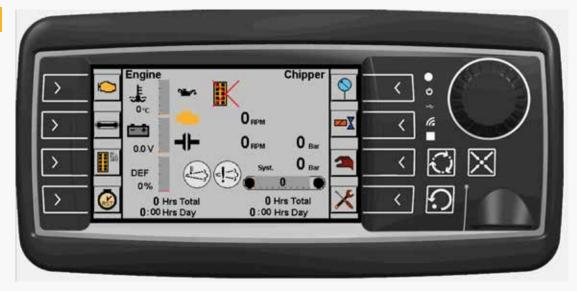
Optionally you can add the Europe Controller with PLC. The revolutionary PLC displays all sorts of relevant information on the performance of the machine. The Europe Controller in combination with proportional valves gives vario chip: You can make chips from G10 to G50, just by pressing one button
